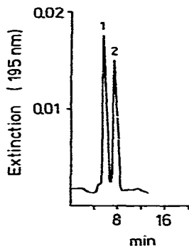
Fig. 2. Elution profile of a Neu5Ac (1) and Neu5Gc (2) mixture (each 200 ng) from anion-exchange HPLC. The mobile phase was 0.75 mM sodium sulphate and the flow-rate 0.5 ml/min at 15 bar. The sialic acids were monitored at 195 nm by 0.04 a.u.f.s. and attenuation 10 mV.
